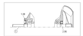
Figure 28: Shaft seal
