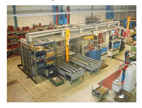
CNC shaft machining centre with gantry equipment
